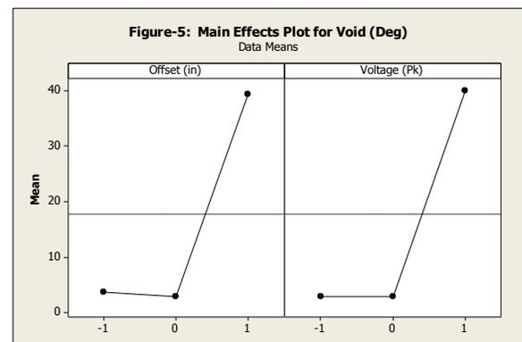
The optimized welding parameters represent Offset and Voltage parameters with a “0” value.
