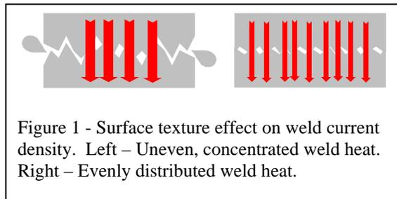
Figure 1 - Surface texture effect on weld current density. Left – Uneven, concentrated weld heat. Right – Evenly distributed weld heat.
