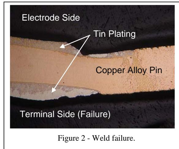
Figure 2 - Weld failure.
