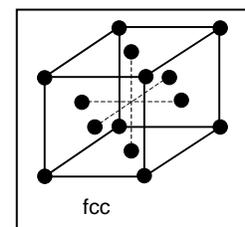
high number of dislocation slip systems in the fcc cubic structure. Group 1 metals can be very hard to weld because of their high thermal and electrical conductivity. Group 1 metals always form a solid state bond with Groups 1, 2, and 3. Note that a solid state bond can still produce a “nugget” or metal button when tensile tested. This phenomenon has sometimes been misinterpreted as a fusion weld.
