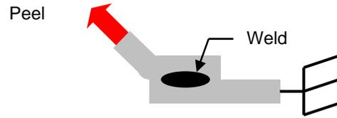
Peel testing applies force to a “narrow strip” of weld contact area. As peeling proceeds, this “narrow strip” breaks away, resulting in the peel force being applied to the “next narrow strip” of contact area.
