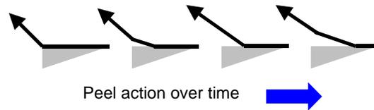
Peel testing disadvantages include large weld strength variances due to variations in: a) weld joint contact area during peeling, b) peel geometry, c) length of the welded assembly, d) amount of the welded assembly in each gripper, and e) material properties of the welded parts such as brittleness.
