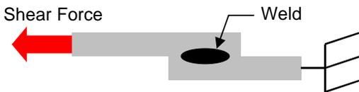
“Stress” is equal to shear force divided by the welded assembly’s cross sectional area. Using “stress” helps to normalize tensile/shear results between welded assemblies with varying cross sectional areas. From a practical viewpoint, it is very hard to measure the effective cross sectional area, so most small-scale weld strength testing relies on just recording the peak force where the part breaks.
