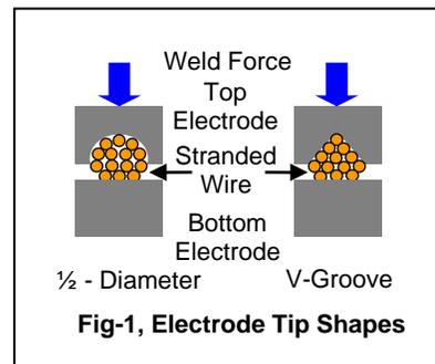
soldering process. Fig-1 shows an opposed electrode configuration, but this process also works with the parallel gap electrode configuration. IMPORTANT - Shaped electrodes will NOT prevent all wire strands from separating from the main wire bundle.
