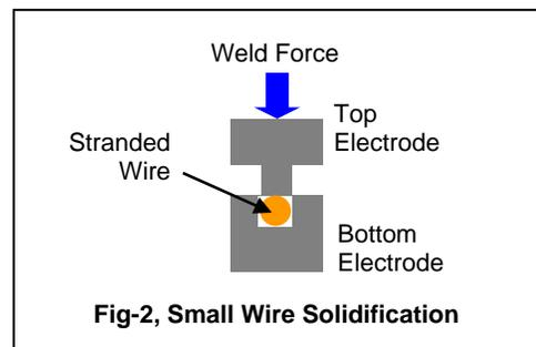
The final solidified wire mass can then be resistance welded to a terminal using a rectangular or round, flat tip electrode. The flat tip is easy to clean, which is a major advantage of this method. Two welding systems are required, one to solidify the wire and a second system to weld the solidified wire to the terminal. The two welding systems represent a minor disadvantage.
