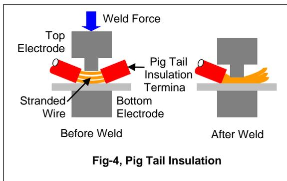
Fig-4, Pig Tail Insulation
