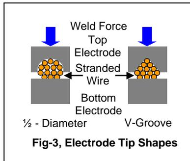
Fig-3, Electrode Tip Shapes
