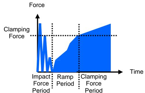
This graph represents weld force versus time for a weld head with impact and clamping force control.
