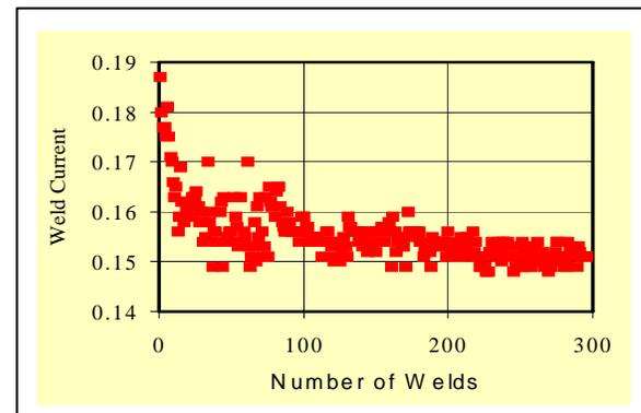
After many welds, the electrode tip surface eventually becomes so heavily pitted, oxidized, and covered with part plating and part material that the heat generated in the weld is adversely affected, resulting in degraded weld strength.
