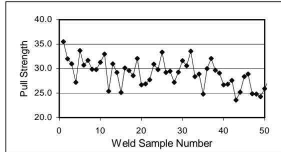
The second welding application shows that electrode seasoning does NOT affect the weld strength and therefore electrode pre-seasoning is not necessary.
