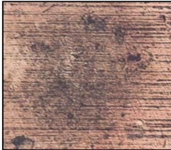
The last photo shows both nickel build-up and copper pitting on the electrode tip face after 100 welds.
