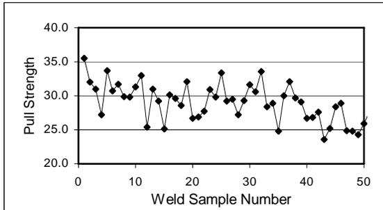
Other parts may be sufficiently thermally robust so that the electrode seasoning process has no effect on the welded parts. See graph below.
