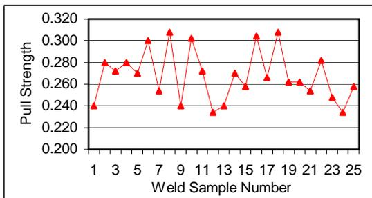
Pre-seasoning the electrodes helps to create a more stable electrode-to-part interface condition, slowing the typical drop off in weld strength with each new weld.
