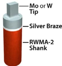
Also, avoid using Mo and W tips that are pressed into a RWMA-2 or Glidcop shanks. Under high weld current and duty cycle operating conditions, the electrical resistance between the shank and tip increases over time, negatively affecting the weld quality.
