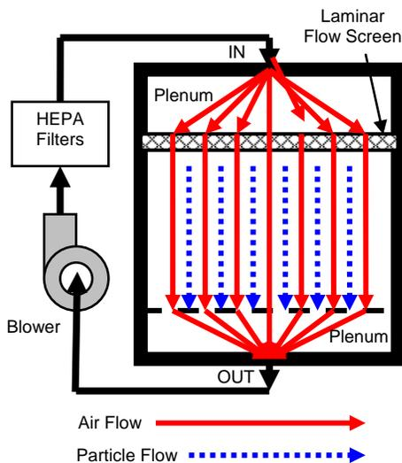
Federal Standard 209E establishes standard classes of air cleanliness for airborne particulate levels in clean rooms. “Class” represents the number of 0.5-micron or larger particles per one cubic foot. The lower the “Class Number”, the fewer the permitted particles per cubic foot<sup>1</sup>. Medical device clean rooms are predominately Class-10,000, although a limited number of Class-1,000 clean rooms exist. Molecular contamination requirements are captured in MIL-STD-1246.
